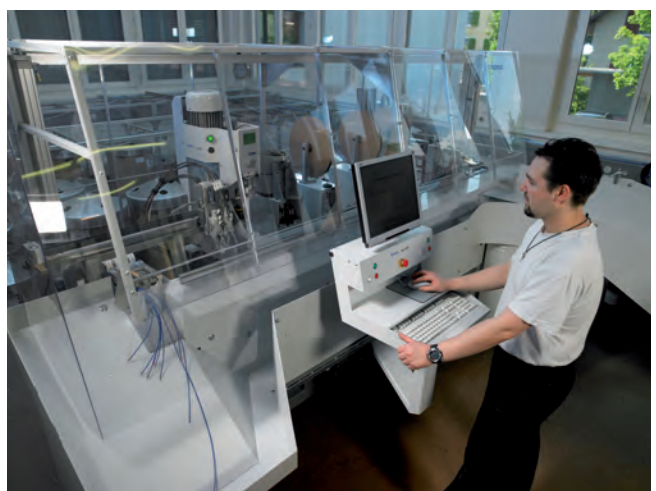
The Zeta 633 is the only machine capable of processing 36 wires simultaneously.
