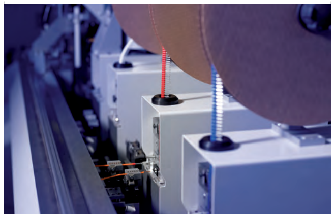
Production of complex wire sequences at the press of a button
