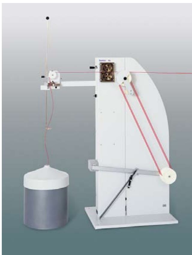
Figure 1: k106 pre-processing station for gentle wire feed
