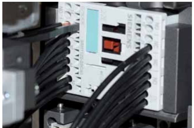
Fully automatic insertion of spring-loaded components
